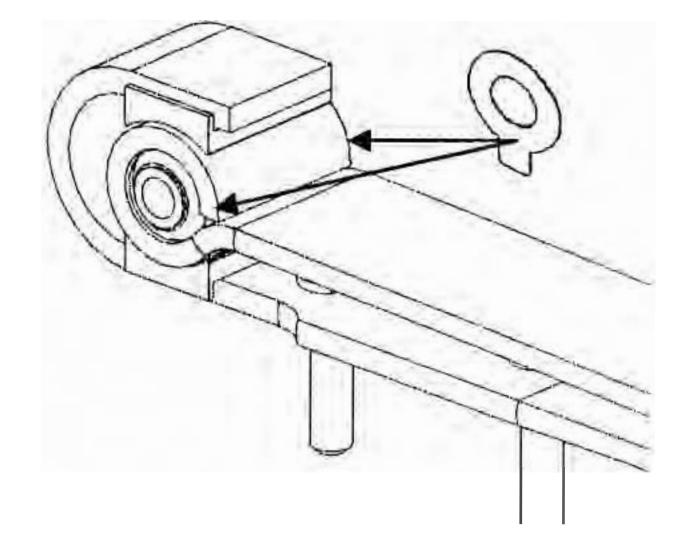
Step 8: place the plastic washer on the spring eye. Be sure the washer does not cover any part of the metal inner tube of the bushing. Repeat this step for both sides of both springs (qty. 4 washers).
